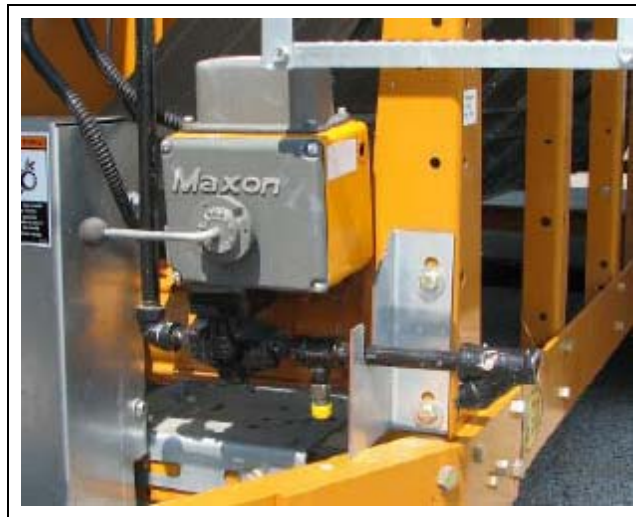
Figure 8C The fuel connection point is equipped with a Y-strainer and Maxon safety valve.
