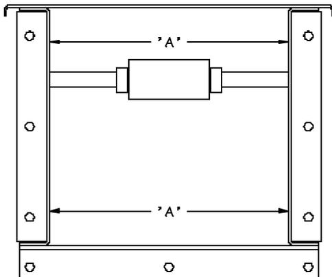
**It is critical for straightness of conveyor that the sides and bottom flanges are aligned flush.** After making sure the flanges are aligned, tighten all hardware on the trough section. When any optional Abrasion Resisting (A.R.) liners are ordered, they may be installed with the 3/8" flat countersunk hardware provided. Adequately tighten liners to conveyor sides. Check that the countersunk hardware is not protruding above the surface of the A.R. liners.
