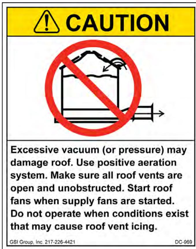
**ATTENTION:** Decal shown below must be present on the outside of the door cover of the two ring, 24 in. (61 cm) porthole door cover and the roof manway cover. If a decal has been damaged or is missing in any of these locations, contact the manufacturer for a free replacement decal.
