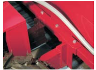
Tractor Frame Bolted to Sweep Assembly.
