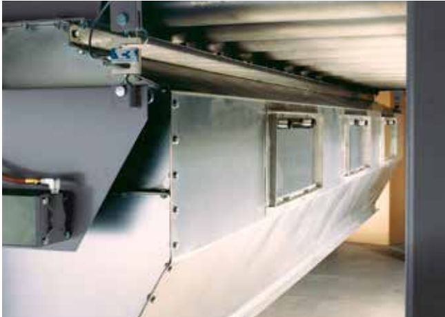
Access doors on the shroud are provided to allow easy cleaning and inspection of the weigh hopper.
