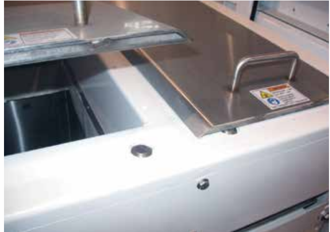
Proximity switches ensure exact current weight is being measured.
