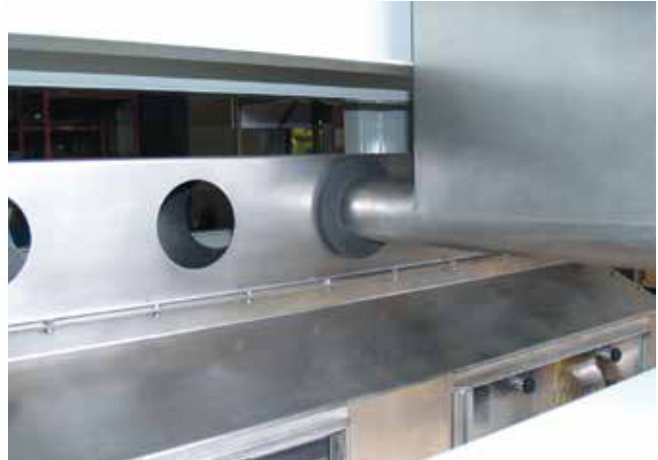
A feeder manifold with dust seals is provided for the top of the weigh hopper shroud.
