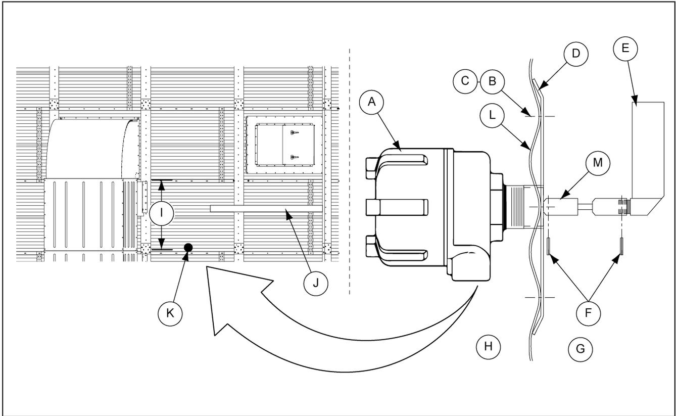
**Figure 5** Storage Chamber High-Limit Rotary Switch (TAF-6106)
