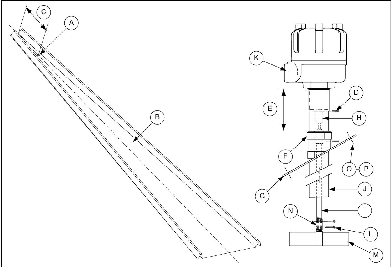
**Figure 2** Drying Chamber High-Level Rotary Switch - Adjustable
