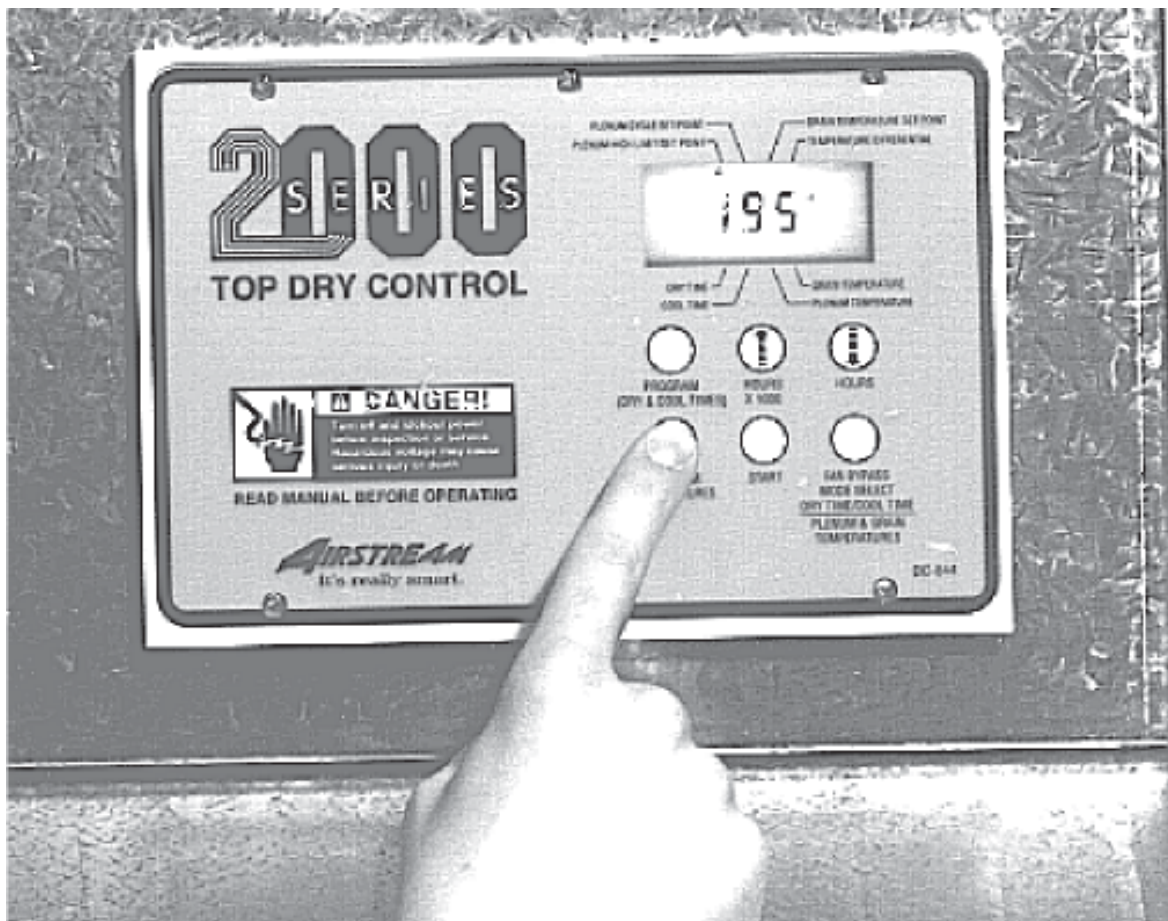
Setting the plenum hi limit on the control box.
