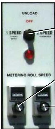
Unload Switch to 2 speed position
