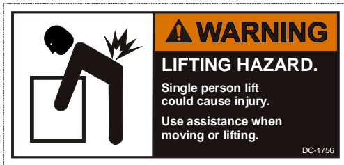
A) DC-1756 Location: Corners of mounting plate. Size: 4 3/4" x 2 1/4"
