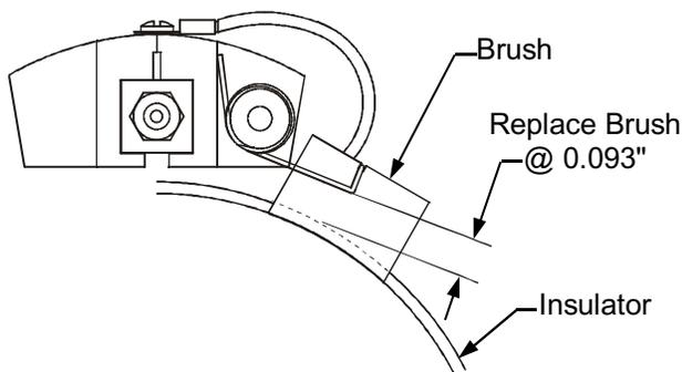
2. Inspect brush contact surface by removing the brush. Remove surface dirt, oxidation, pitting, or other contaminants (with a wire brush).
