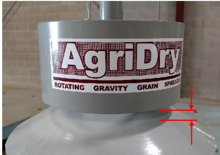
FIGURE 54. DISTANCE LEVELING BAND IS OFF CONE
