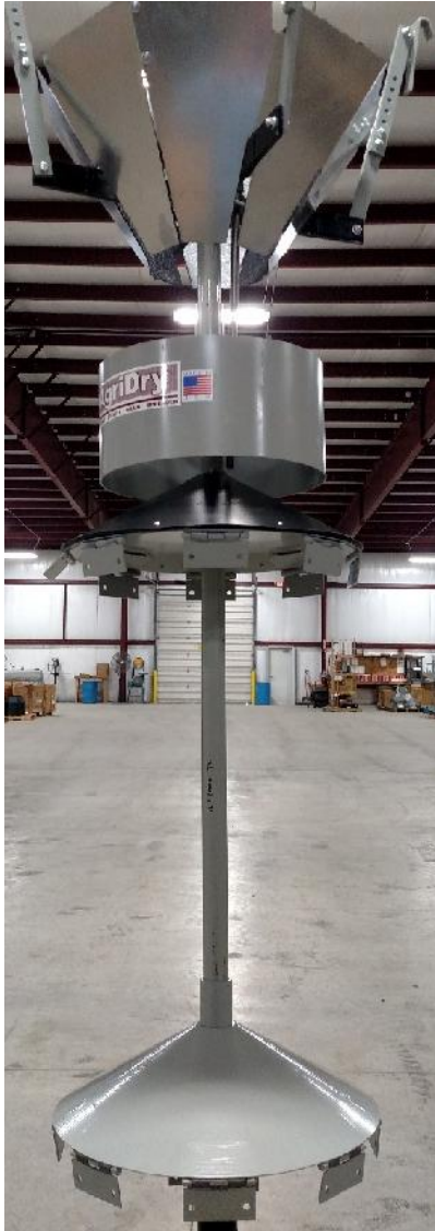
FIGURE 28. CONE AND SPACER LOWERED
