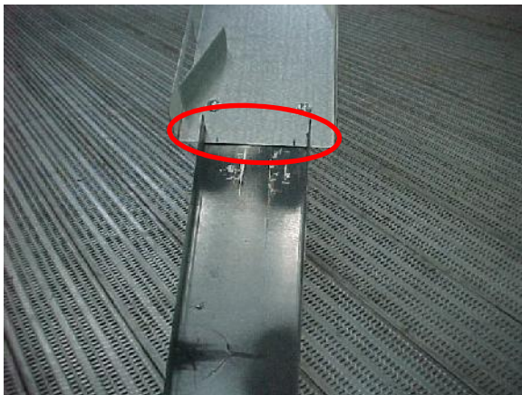
FIGURE 36. EXTENSION CHUTE FLANGES OVER BOTTOM CHUTE
