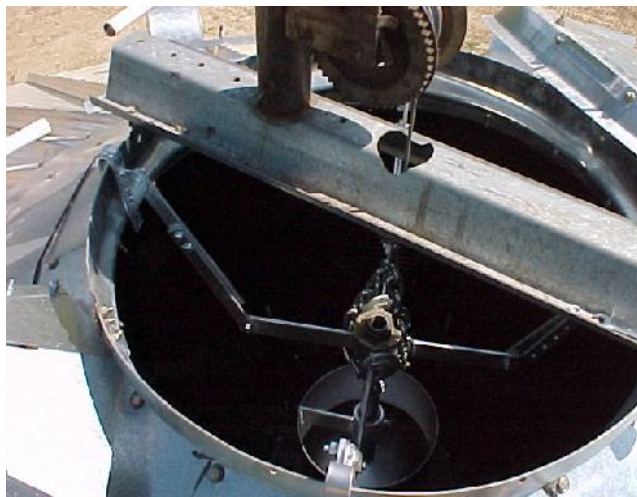
FIGURE 44. SPREADER HANGING FROM PEAK RING
