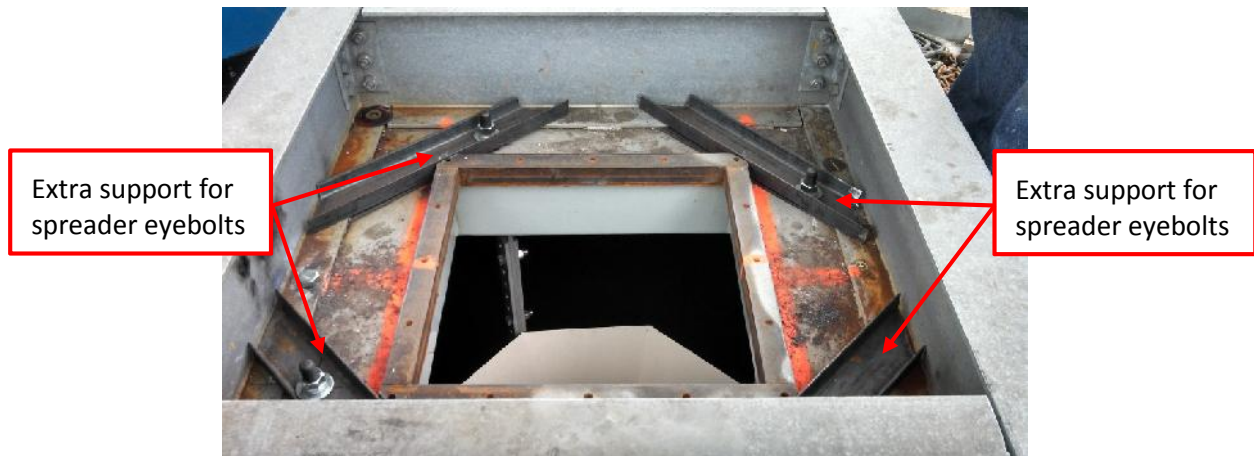
FIGURE 50. SPREADER EYEBOLTS MOUNTED IN "C" CHANNEL SUPPORTS
