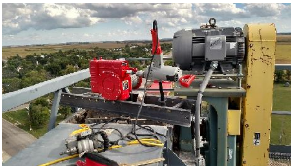
FIGURE 2. WORM GEAR WINCH W/POWER DRILL
