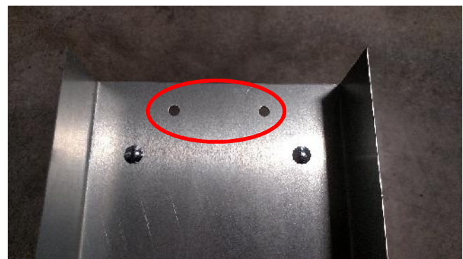
FIGURE 16. MOUNTING HOLES FOR CENTER SHAFT HINGE
