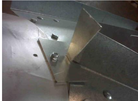
FIGURE 38. ASSEMBLED FILLER CLIP
