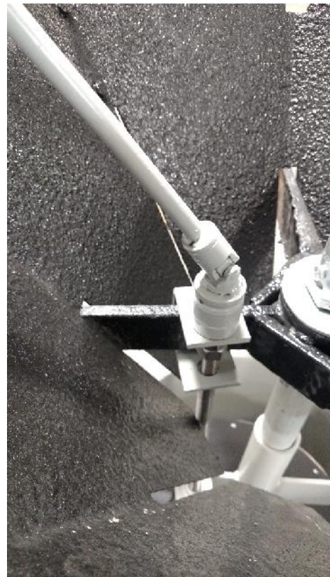
FIGURE 55. UNIVERSAL ADJUSTMENT ROD ON THE ACME THREAD
