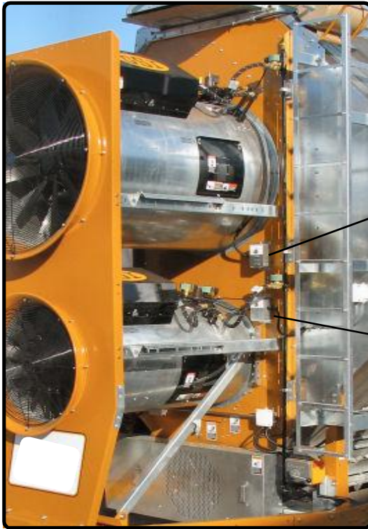
Air Switch locations.
