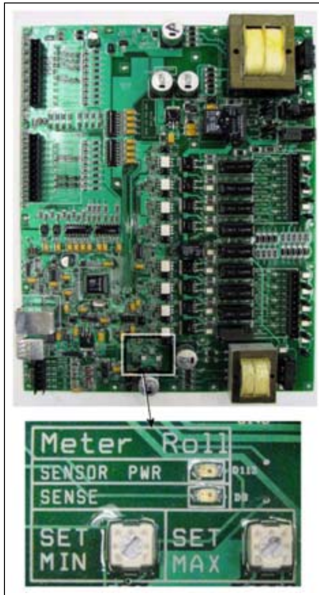
Figure 3D Main I/O Board with a Close Up View of the Set Minimum and Set Maximum Potentiometers
