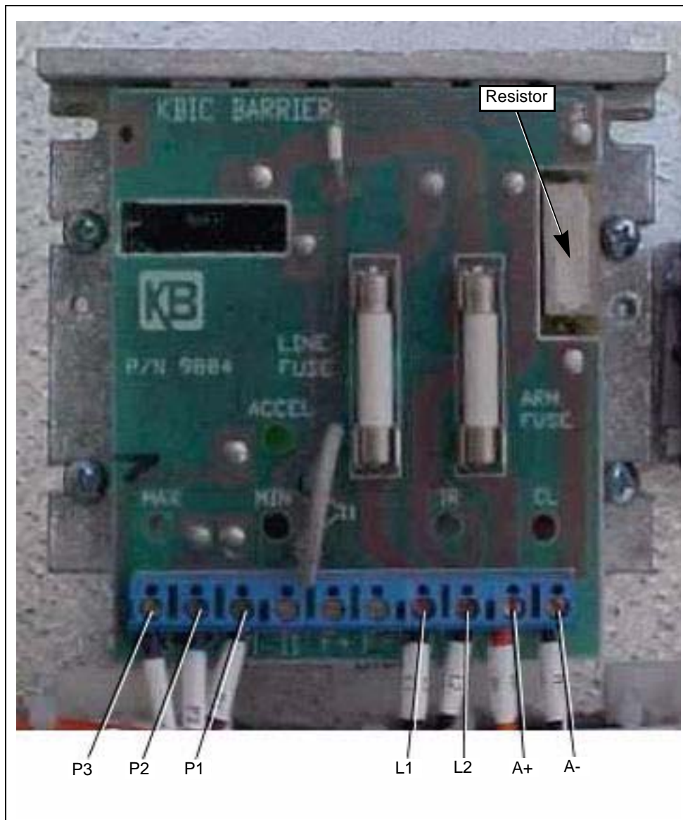
Figure 1C SCR Board Terminals
