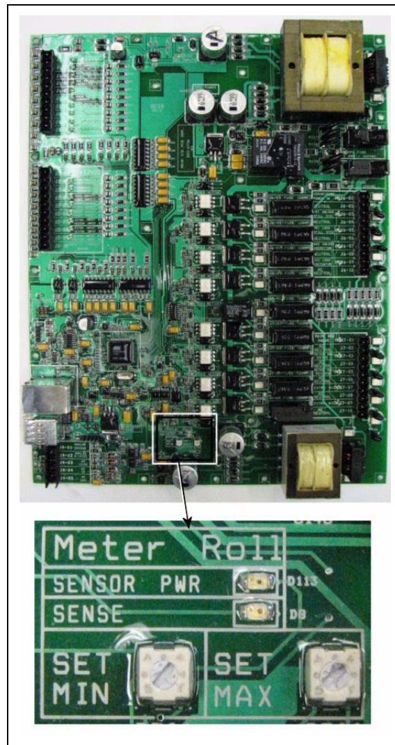
Figure 3A Main I/O Board with a Close Up View of the Set Minimum and Set Maximum Potentiometers
