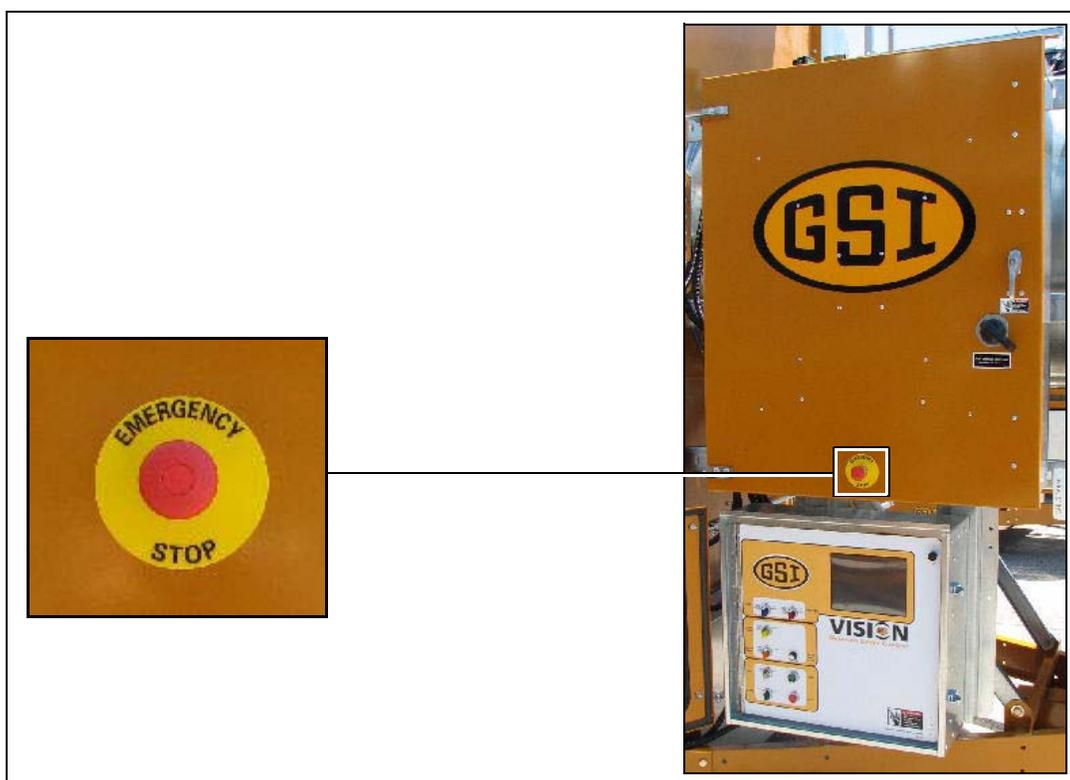
The Emergency Stop switch is located on the upper control box door. Pushing the Emergency Stop switch will interrupt the control power and stop all dryer functions.
