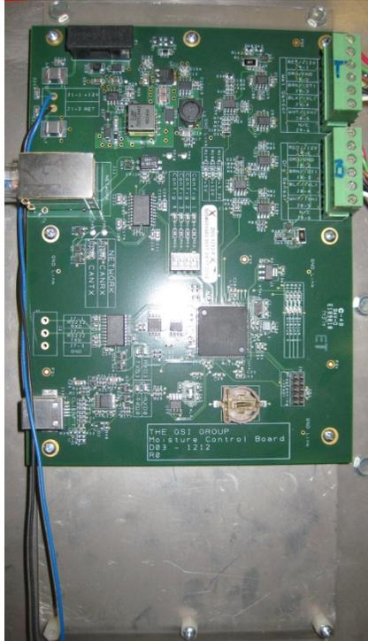
Fig. 2 New Style Moisture Control Board Installed
