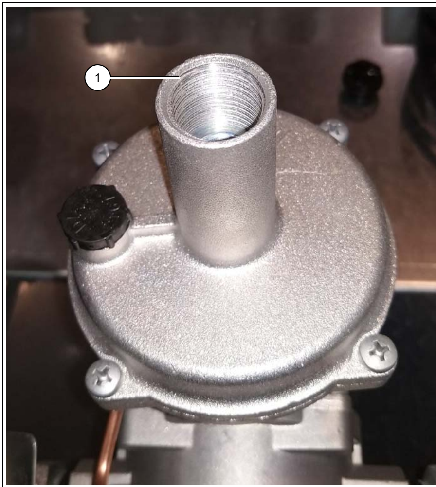
Figure 5B Over Pressure Safety Valve
