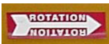
Part Number: DC-219 Located on fan inlet cone.
