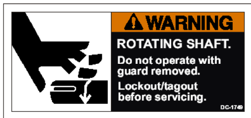
Part Number: DC-1749 Size: 1.75" x 3.75" Located on fan coupling guard on motor driven fans.
