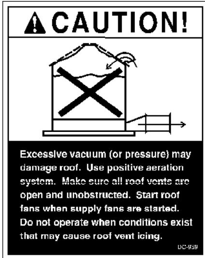
GSI DOES NOT WARRANT ANY ROOF DAMAGE CAUSED BY EXCESSIVE VACUUM OR INTERNAL PRESSURE FROM FANS OR OTHER AIR MOVING SYSTEMS. ADEQUATE VENTILATION AND/OR "MAKEUP AIR" DEVICES SHOULD BE PROVIDED FOR ALL POWERED AIR HANDLING SYSTEMS. GSI DOES NOT RECOMMEND THE USE OF DOWNWARD FLOW SYSTEMS (SUCTION). SEVERE ROOF DAMAGE CAN RESULT FROM ANY BLOCKAGE OF AIR PASSAGES. RUNNING FANS DURING HIGH HUMIDITY/COLD WEATHER CONDITIONS CAN CAUSE AIR EXHAUST OR INTAKE PORTS TO FREEZE.
