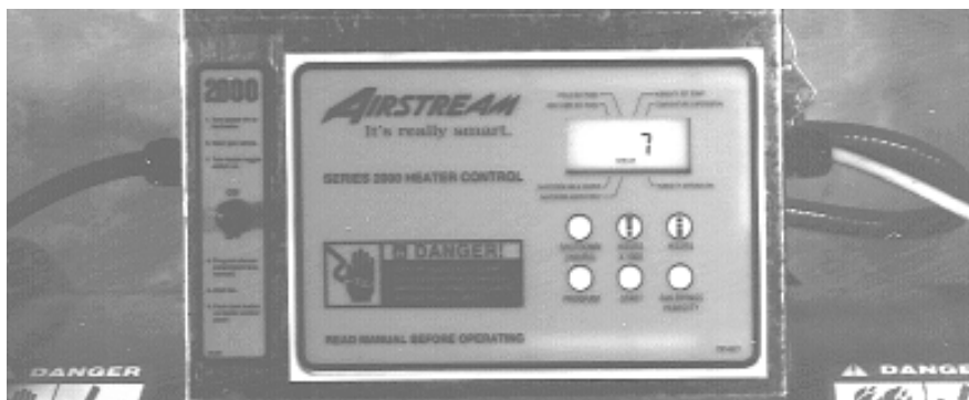
The heater control display showing error #7.
