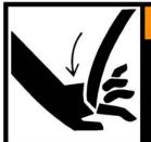
Stay clear of rotating blade. Blade could start automatically. Can cause serious injury. Disconnect power before servicing. DC-1225
