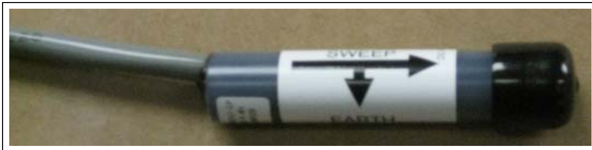
Figure 4AD Accelerometer Assembly Installation
