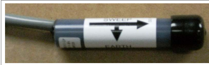
Figure 3 Accelerometer Assembly Installation
