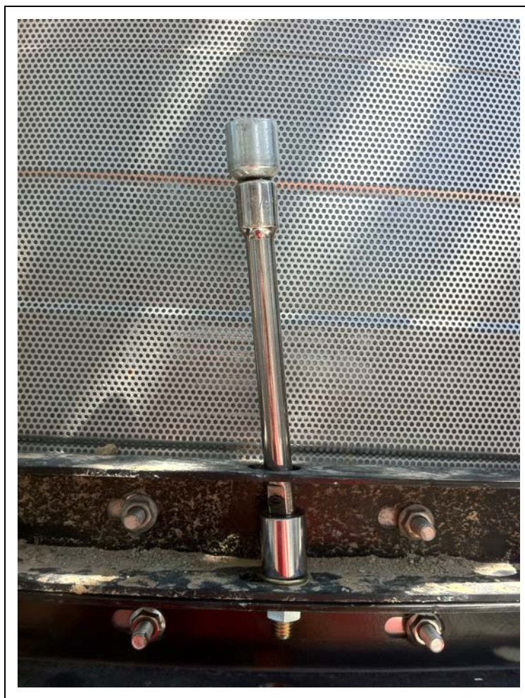
Figure 5D Connecting channels often requires the use of socket extensions. Please plan accordingly.
