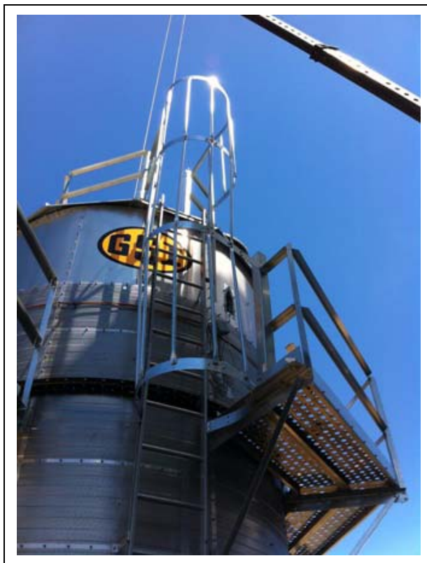
Figure 7B Consider overhead clearance for the entire height of the dryer.
