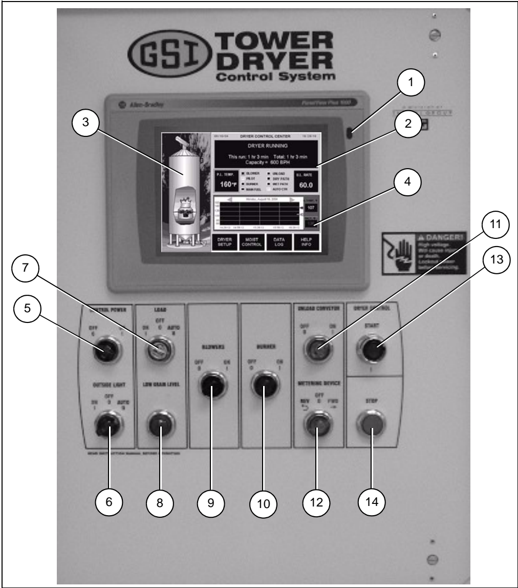
Figure 3H PLC Control Screen
