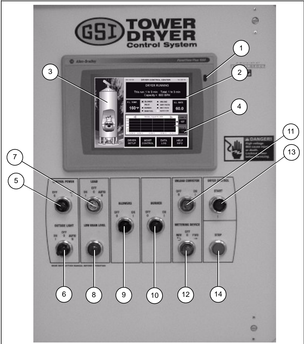
Figure 3H PLC Control Screen
