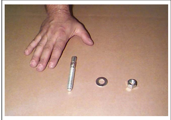
Figure 28C Anchor bolt, heavy duty expanding, 5-1/2"
