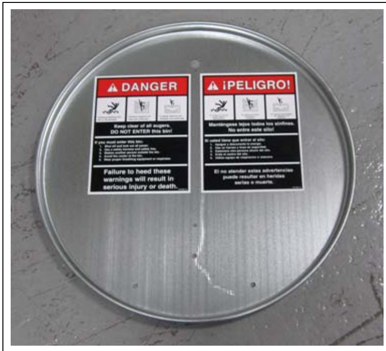
Figure 6AH Access door cover with “DANGER - Avoid Suffocation” decals.
