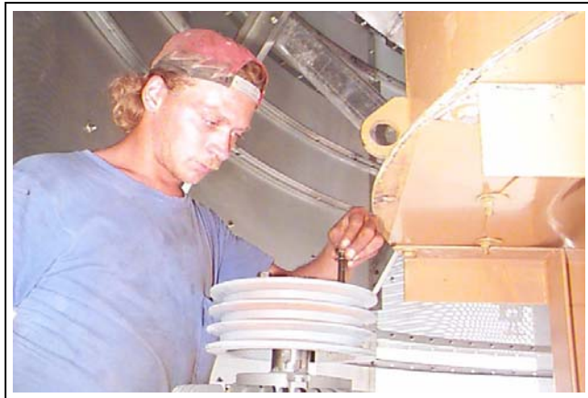
Figure 16Q Inserting motor sheave to motor hub.
