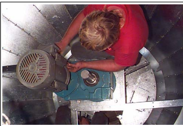
Figure 22Y Bolting motor to gearbox (top mount). NOTE: Motor to gearbox configuration can vary.
