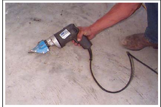
Figure 18D Use metal shear to cut wall sheets and screen.
