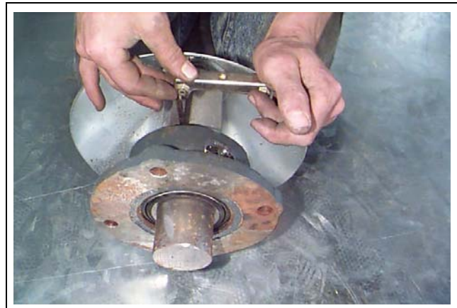
Figure 22M Tightening set screw on metering drum bearing.
