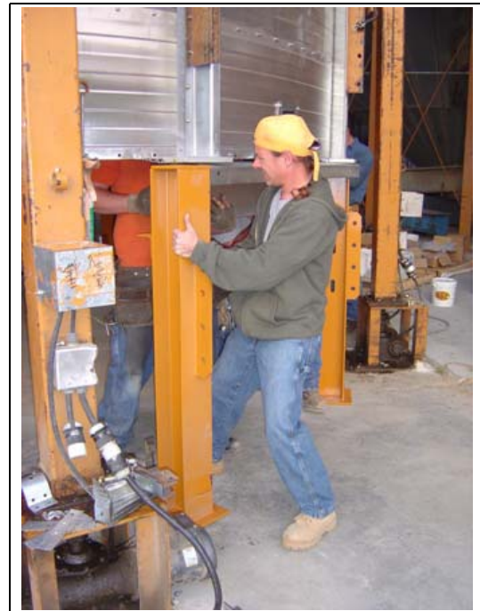
Figure 19R Placing upper leg directly under base stiffener weldment.
