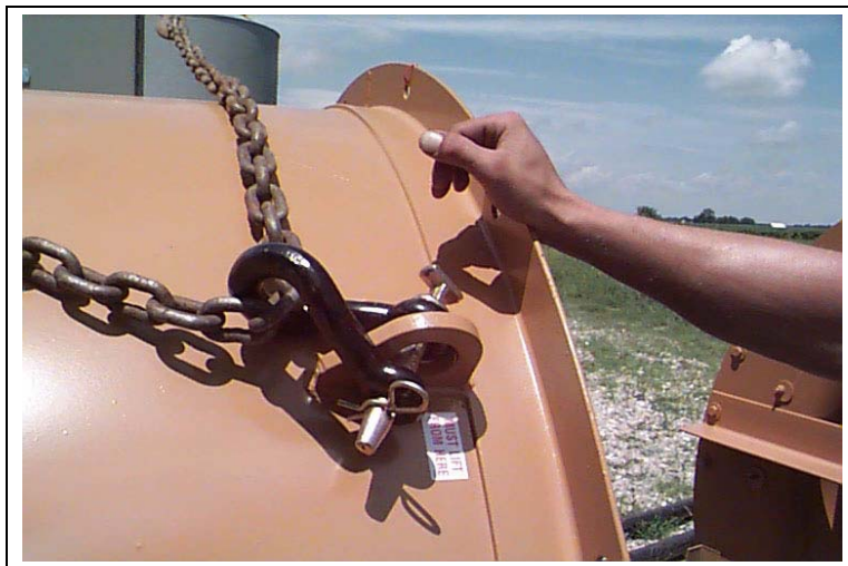
Figure 15S Lifting tackle is attached to fan lift eyelets.
