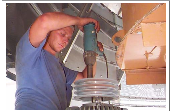
Figure 16X Tightening motor sheave bolts. NOTE: Final tightening of bolts should be with torque wrench.
