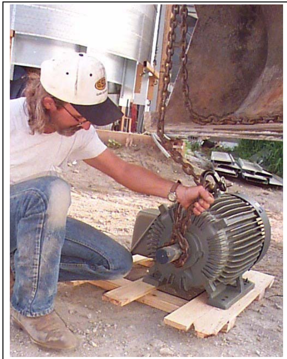
Figure 16H Attach lifting tackle to fan motor.
