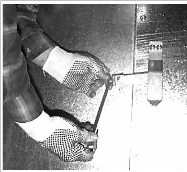
Figure 18AX Adjusting bolt on latch bar.
