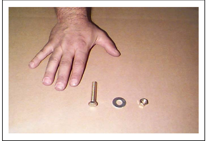
Figure 28N 3/8" x 2" Bolt, Washer and Nut
