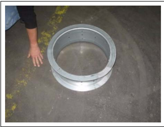
Figure 5AB Plenum Roof Center Collar
