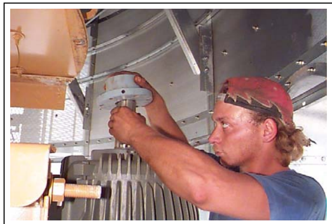
Figure 16N Sliding motor hub on motor drive shaft.
