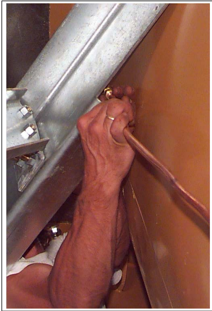
Figure 17J Attaching grease tube to brass compression union.
