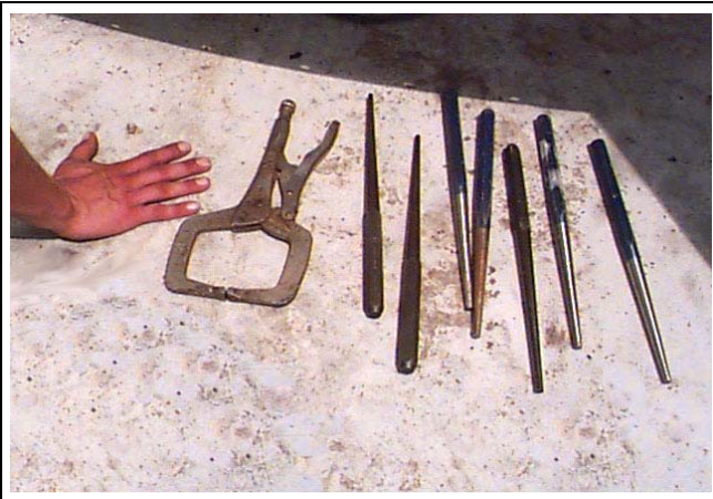
Figure 27A C-Clamp and assorted alignment punches.
