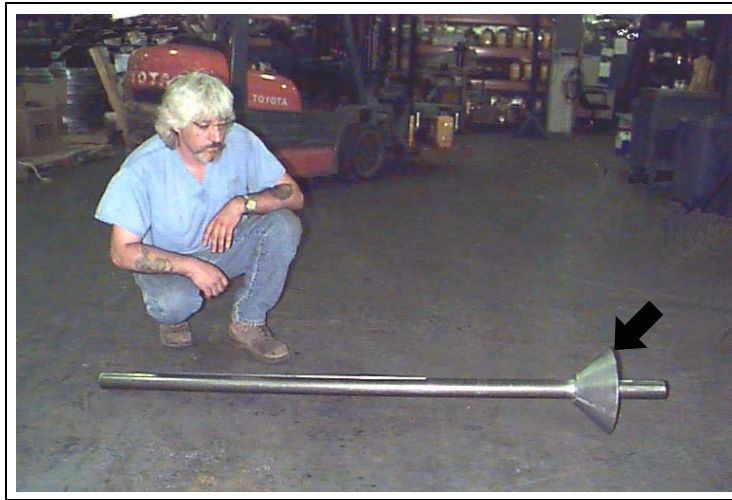
Figure 22G Metering drum drive shaft weldment 6' (2-3/8"). NOTE: Grain deflector (arrow) is over bearing thrust collar.
