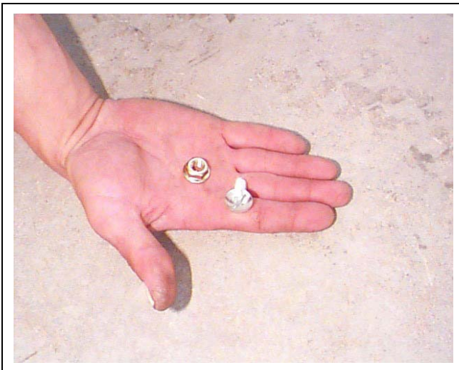
Figure 18C 5/16" x 3/4" Slotted truss head bolt and 5/16" whiz lock nut.
