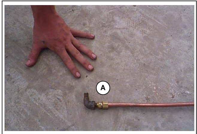
Figure 17C Close Up - Elbow end of grease tube (A).
