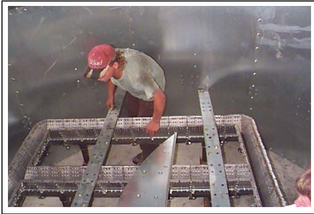
Figure 14H Moving burner, burner baffles and other parts inside burner housing.
