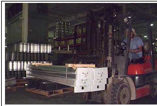
Figure 19H Base stiffener weldments as shipped.
