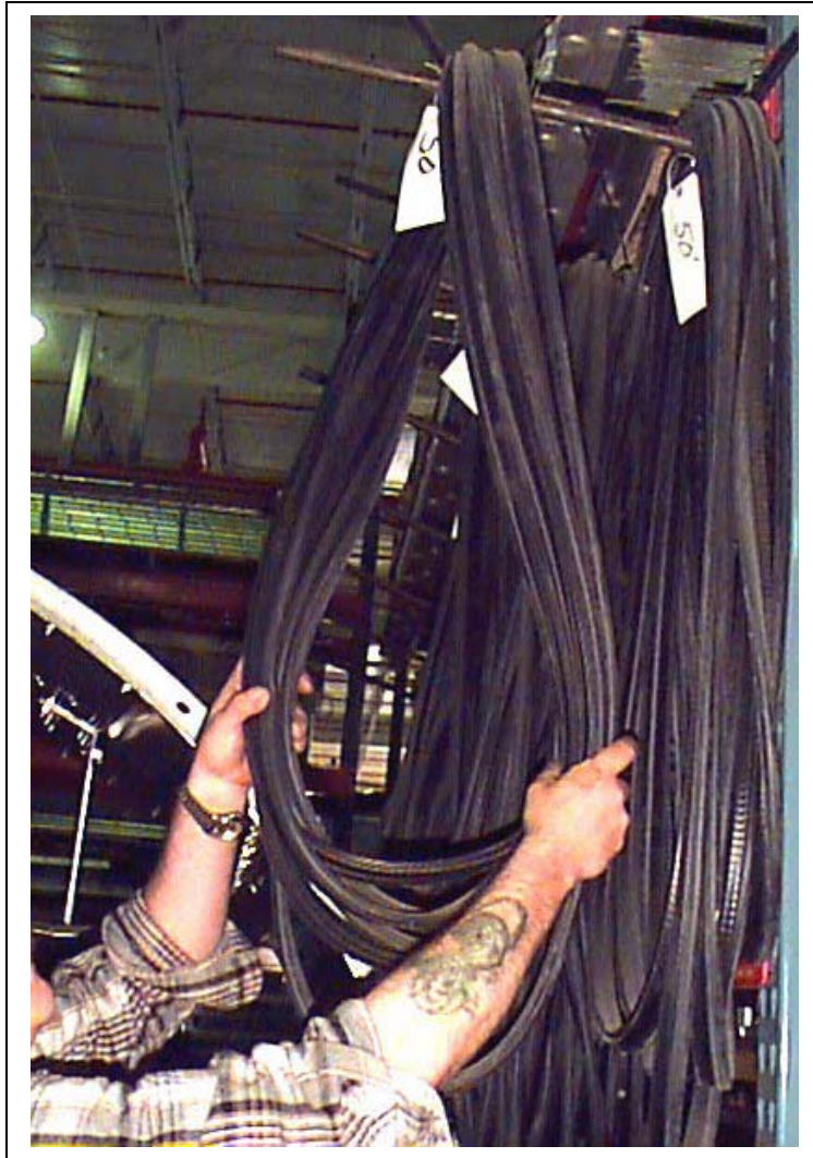
Figure 6F Bulb seal as shipped.
