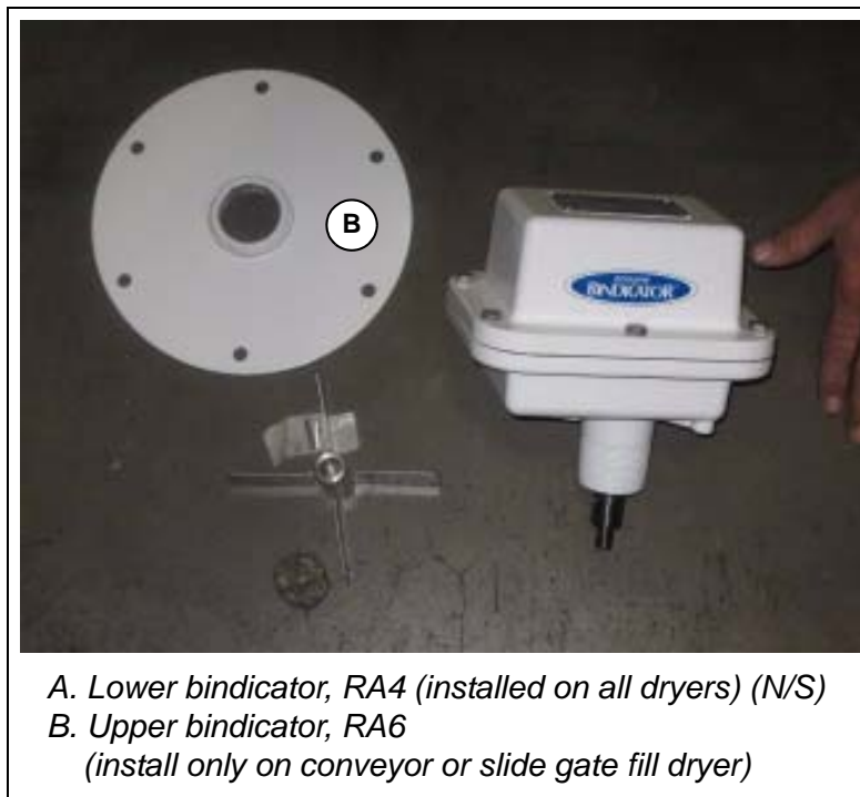
Figure 8H Bindicators (wired for demonstration)
