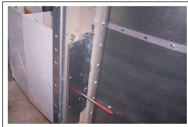
Figure 13B Close Up - Grain Turner Offset Bracket (Symmetrical - There is no up or down)
