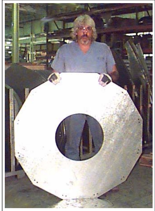
Figure 21I Metering Drum Floor
