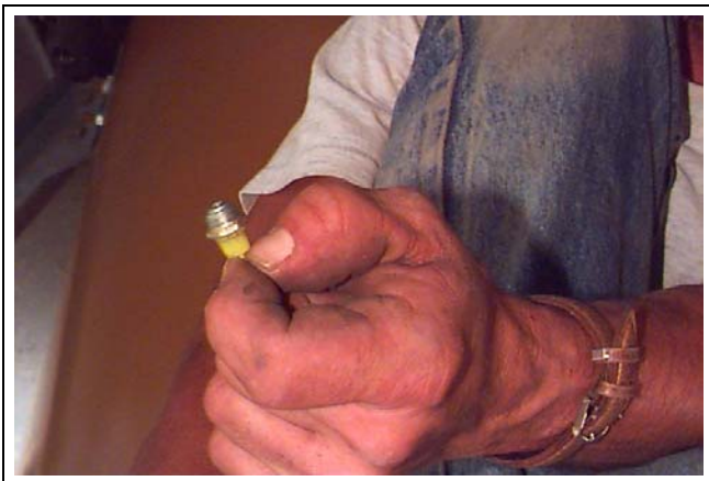
Figure 17G Grease zerk removed from fan.
