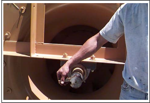
Figure 15R Remove fan drive shaft key and save it. (Do not discard.)
