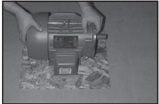
Photo 20-2 Metering Drum Motor as shipped.
