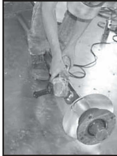
Photo 20-15 Cleaning Metering Drum Drive Shaft Weldment.
