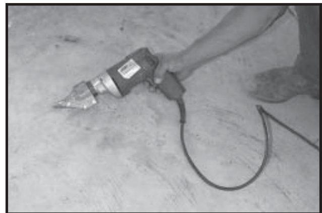
Photo 16-4 Use Metal Shear to cut Wall Sheets and screen.
