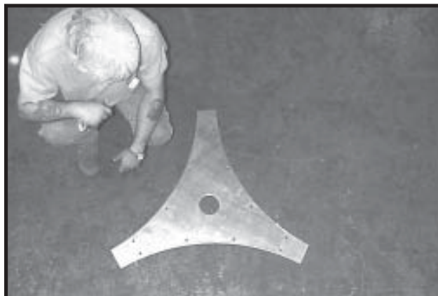
Photo 13-3 Fan Housing Splice.
