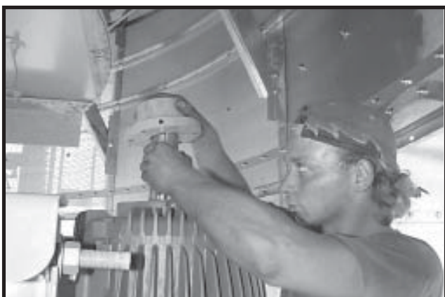
Photo 14-14 Sliding Motor Hub on Motor Drive Shaft.
