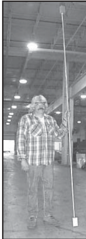
Photo 5-21 A pair of RTDs on (1) 10' length of conduit. Note either RTD on conduit can be installed in top position.
