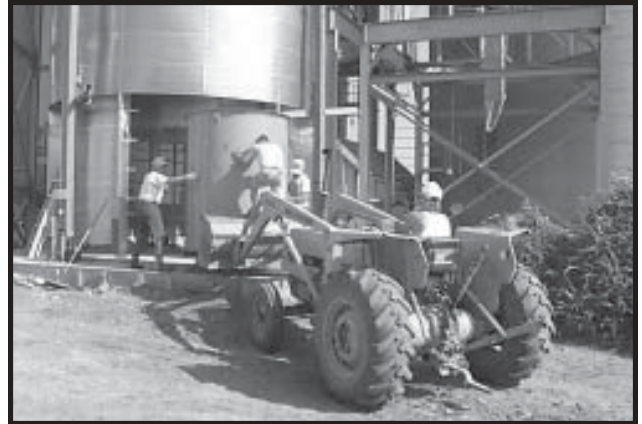
Photo 13-18 Pushing Fans into dryer.
