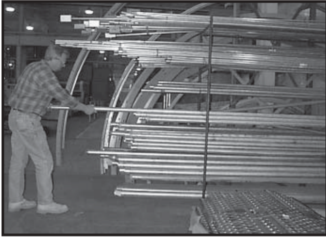
Photo 5-1 1/2" IMC rigid, threaded conduit.
