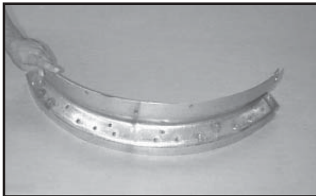
Photo 3-12 Tower Roof Center Collar Section (1 of 3).
