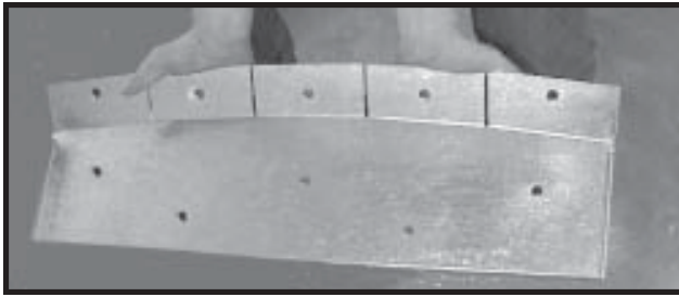
Photo 19-5 Inside Hopper Flange.
