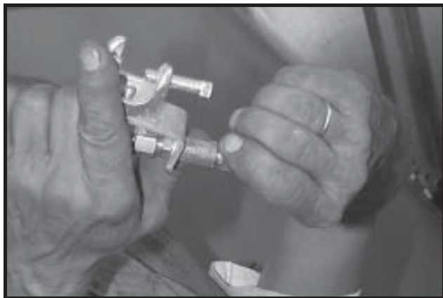
Photo 15-8 Screwing Grease Zert into coupling on Beam Clamp end of Grease Tube.
