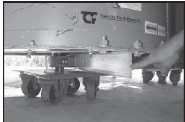
Photo 13-16 Close up - Fan with Drive Shaft down on dolly.
