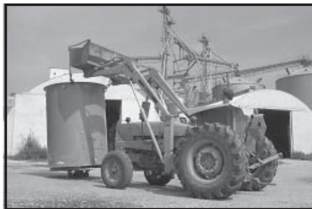
Photo 13-15 Stand Fan up vertical with Drive Shaft down on dolly.
