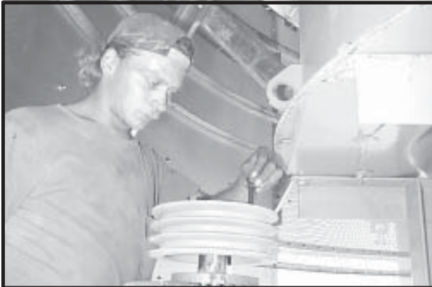
Photo 14-17 Inserting Motor Sheave to Motor Hub.
