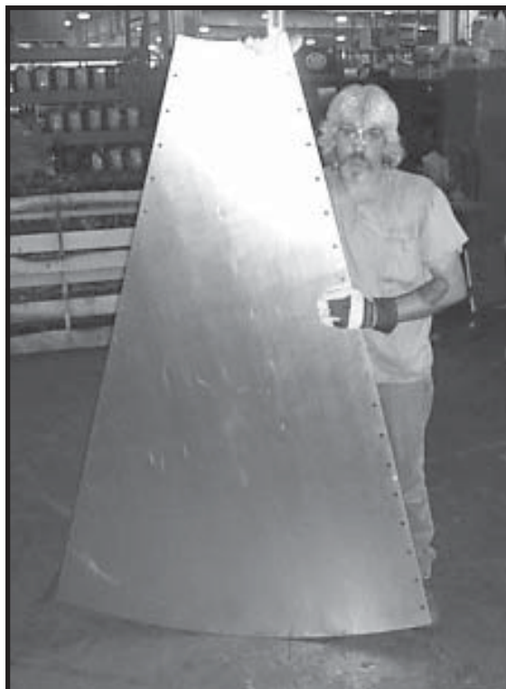
Photo 18-3 Cool Section Floor Sheet.
