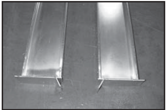
Photo 2-20 Bottom of Plenum Roof Rafters installs to Eave Channel.
