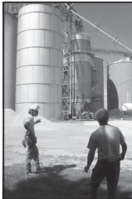
Photo 17-22 Sighting from a distance to check entire length of dryer is vertical.
