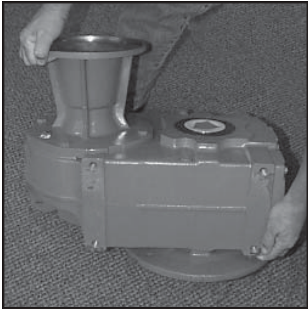
Photo 20-9 Metering Drum Gearbox (90:1).
