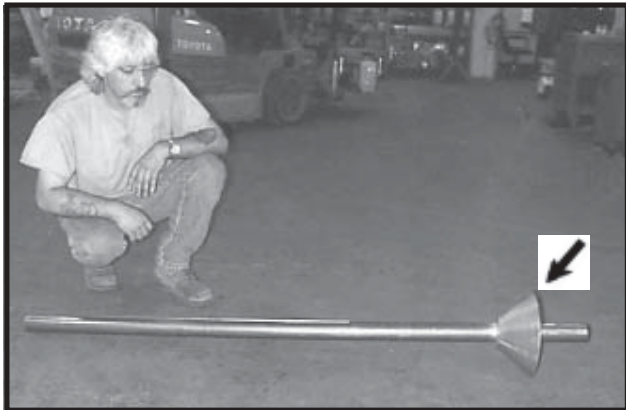
Photo 20-6 Metering Drum Drive Shaft Weldment 6' (2-3/8"). Note Grain Deflector (arrow) is over Bearing Thrust Collar.
