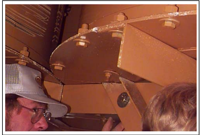
Figure 16D Align fan motor mount and bolt to fan.
