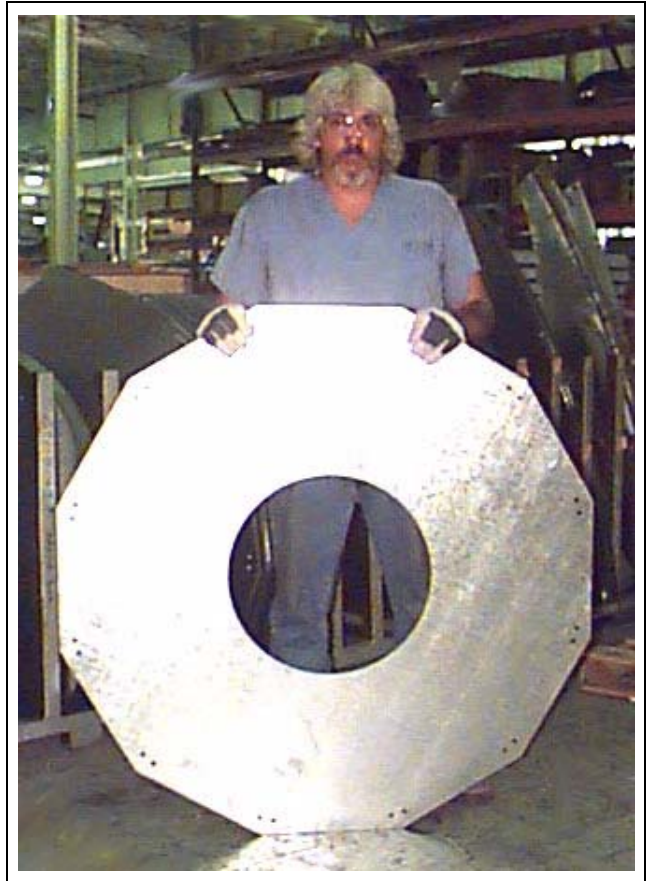
Figure 21I Metering Drum Floor
