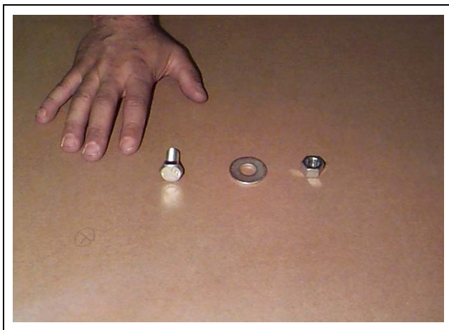
Figure 28H 1/2" x 1" Hex Head Bolt, Washer and Nut
