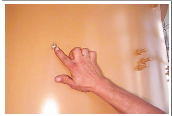
Figure 15AB Close Up - Upper Grease Zerk
