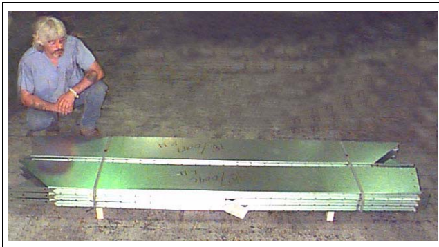
Figure 21D Hopper channels, R.H. and L.H. install with diagonal-cut end down. Bottom side has horizontal flange. Top side has vertical flange.
