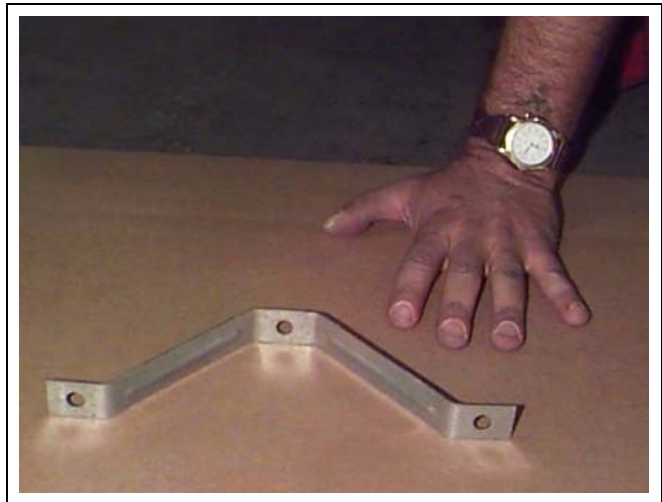
Figure 11C Close Up - Inside ladder standoff.
