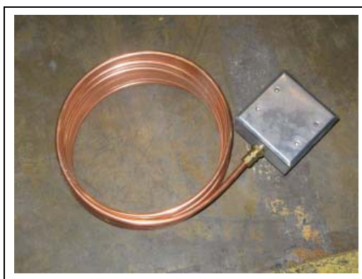
Figure 8N One (1) (outside) High-Limit consists of one (1) junction box and two (2) copper tubings.
