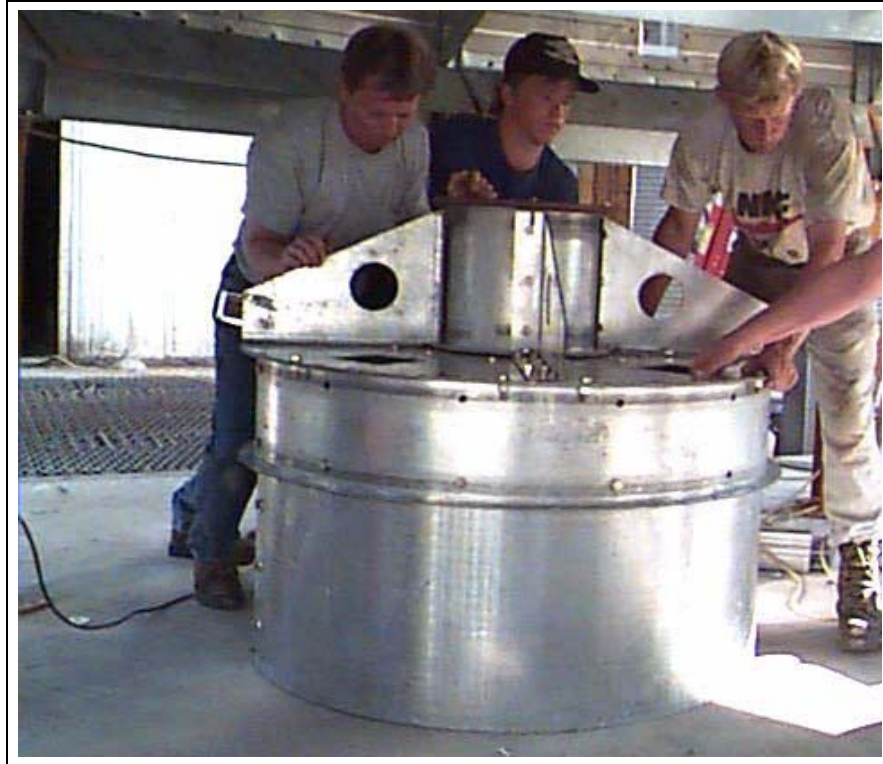
Figure 20B Moving metering drum into center of dryer.
