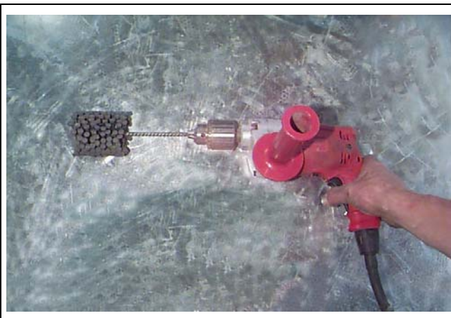
Figure 27C Drill with ball-hone to clean out gearbox bore.
