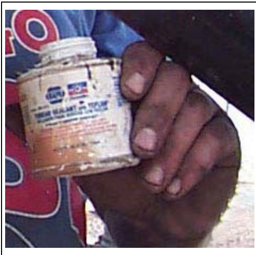
Figure 24M Seal all threaded pipe connections with heavy duty pipe sealing compound.
