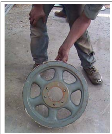
Figure 16M Fan Sheave
