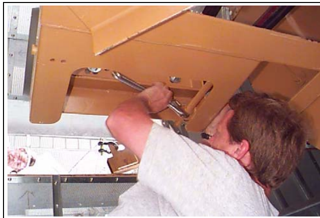
Figure 16AC Once belts have proper tension, tightening adjusting nuts on bottom rod of motor mount.
