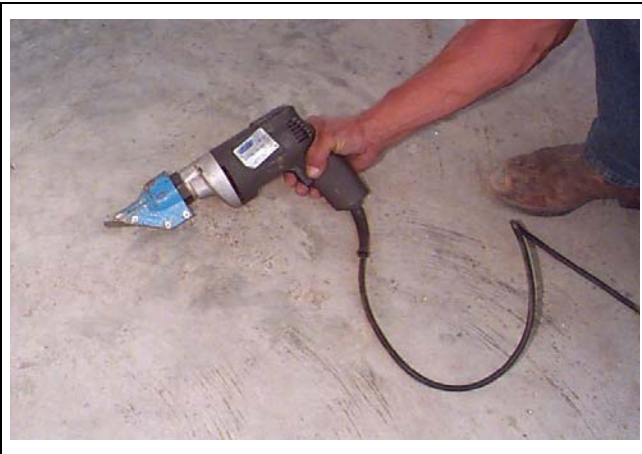
Figure 27B Metal shear to cut wall sheets and screen.
