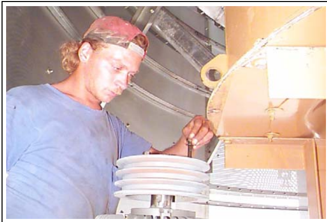
Figure 16Q Inserting motor sheave to motor hub.
