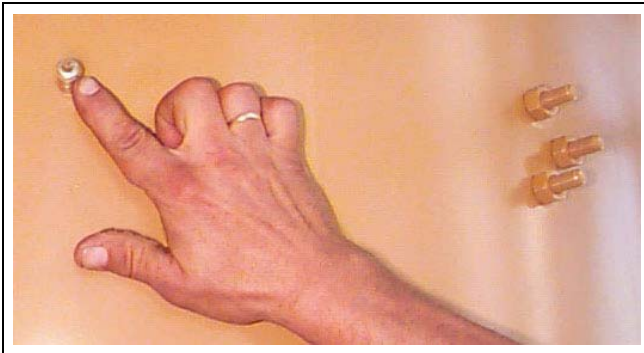
Figure 17A Close Up - Grease zerk on fan.
