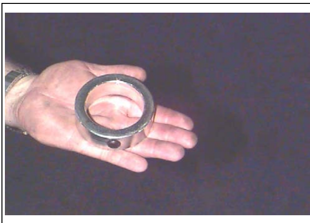
Figure 22I Gearbox Set Collar 2-3/8"
