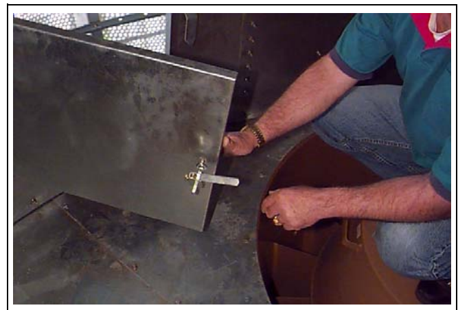
Figure 18BA Reducer door is installed. NOTE: Hinges are on L.H. side in this example.
