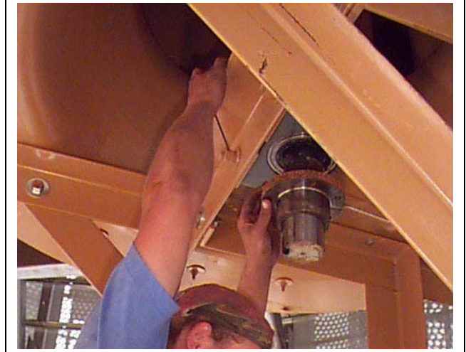
Figure 16R Sliding fan hub on fan drive shaft.
