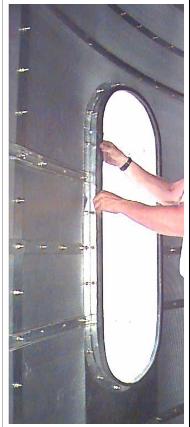
Figure 18AS Pressing bulb seal around inside edge of heat section door sleeve.
