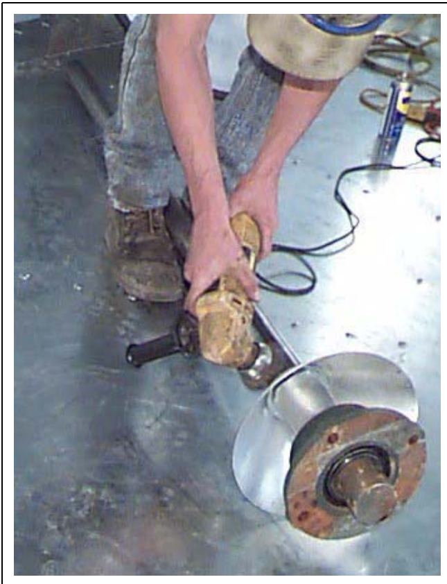
Figure 22L Cleaning metering drum drive shaft weldment.
