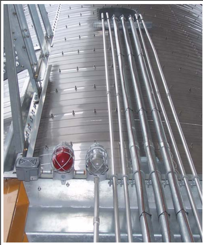
Figure 4S Rear View - Lights and horn installed on 3 fan dryer.
