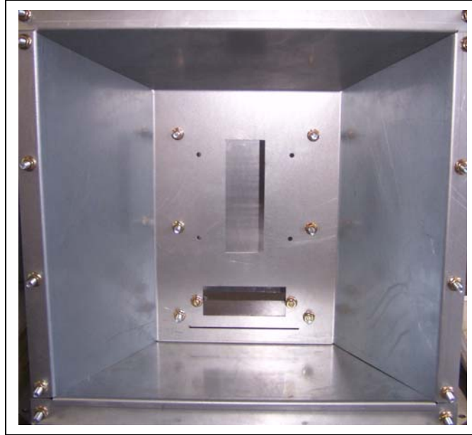
Figure 10AC Dry Moisture Sensor Housing Assembly
