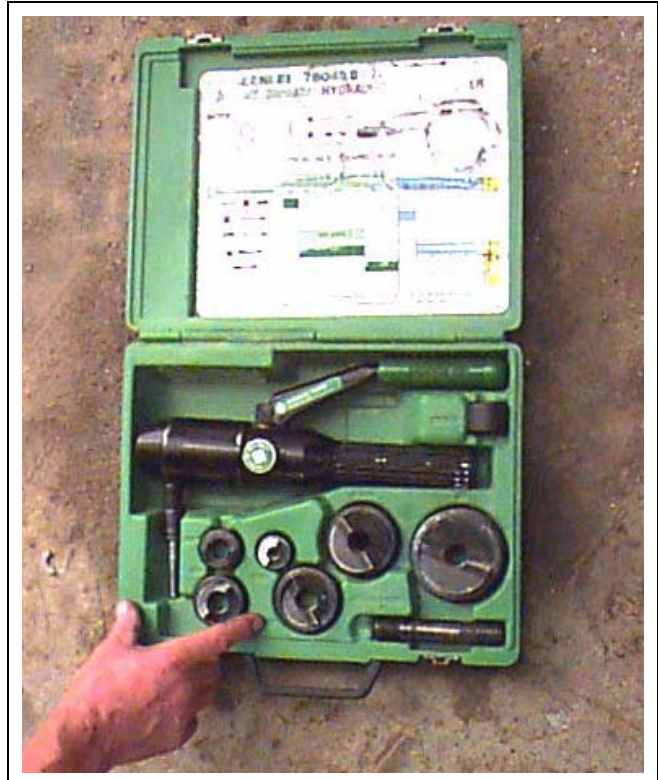
Figure 4U Hydraulic punch driver set with 1/2" to 2" knock out punches.
