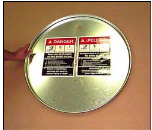
Inside view - Hatch door installed with decals in place.
