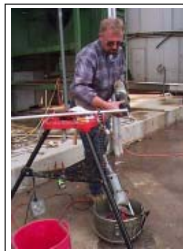
Figure 14B Hand Threader for 1/2" Aluminum Conduit
