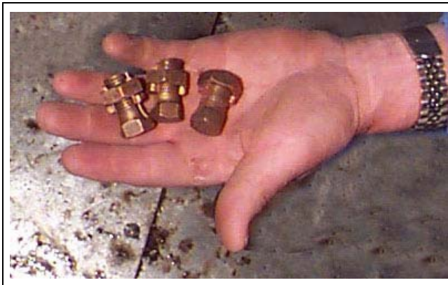
Figure 5E Split Bolt Connectors (6 per fan motor).
