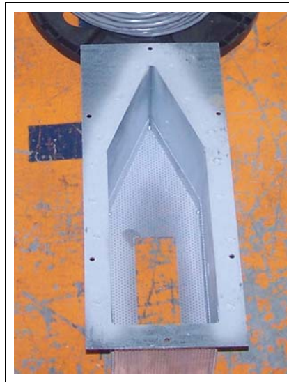
Figure 10W Wet Moisture Sensor Housing
