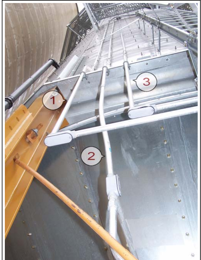
Figure 4S Rear View - Lights and horn installed on 3 fan dryer.
