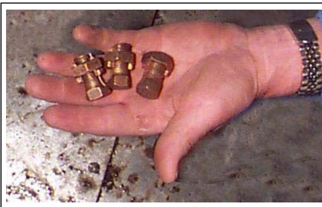
Figure 5E Split Bolt Connectors (6 per fan motor).
