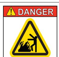
Automatic equipment can start at any time. Do not enter until fuel is shut off and electrical power is locked in off position. Failure to do so will result in serious injury or death.
