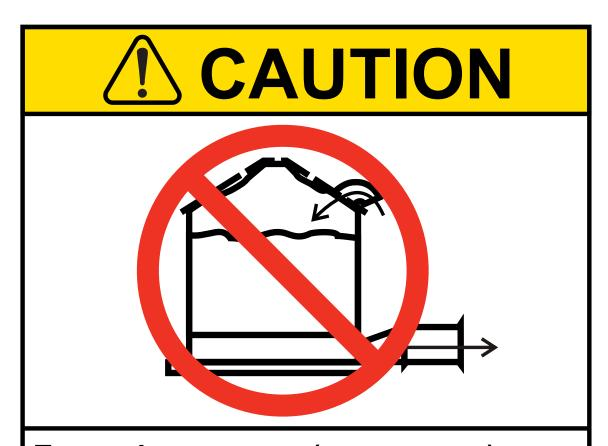
Excessive vacuum (or pressure) may damage roof. Use positive aeration system. Make sure all roof vents are open and unobstructed. Start roof fans when supply fans are started. Do not operate when conditions exist that may cause roof vent icing.
