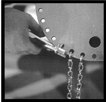
Crimp "S" hooks after final chute adjustment
