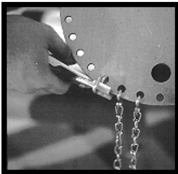
Crimp "S" hooks after final chute adjustment
