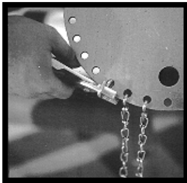
Crimp "S" hooks after final chute adjustment
