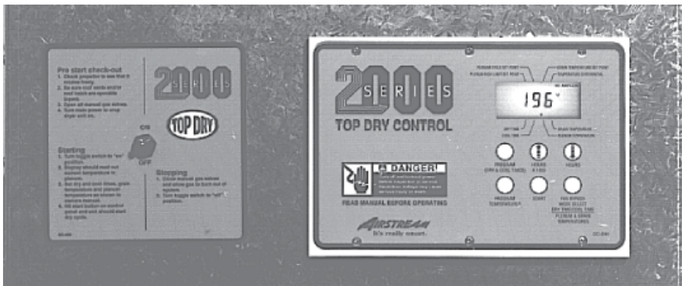
The control panel of the Top Dry heater unit.
