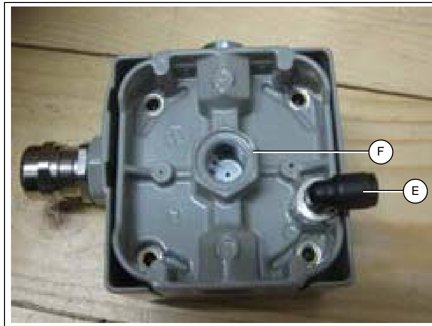
Figure 2H Differential Pressure Switch
