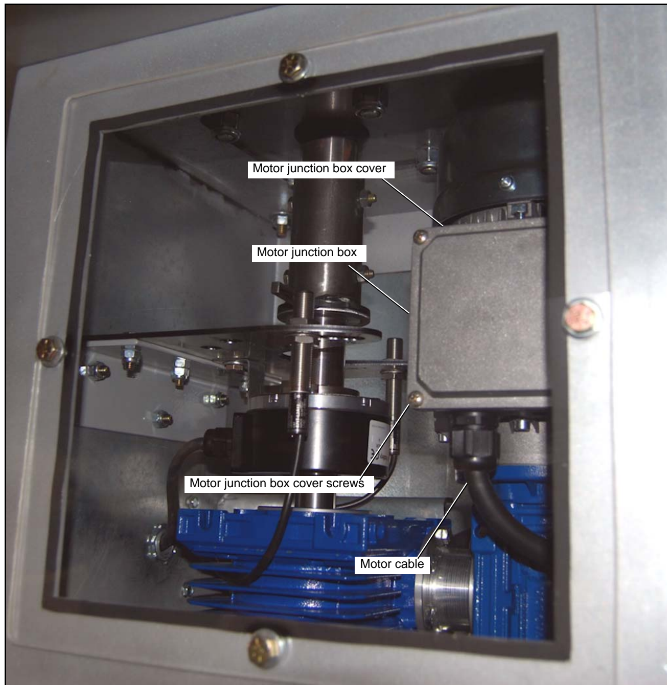
Cable fitting connection to motor junction box
