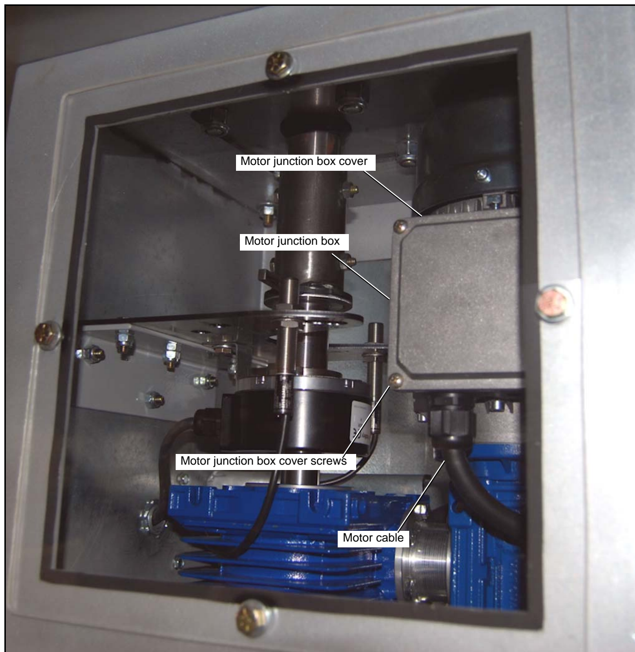
Cable fitting connection to motor junction box
