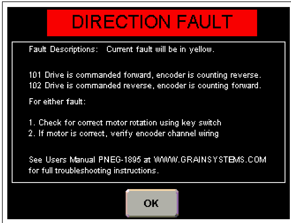
Figure 4Y Direction Fault Screen
