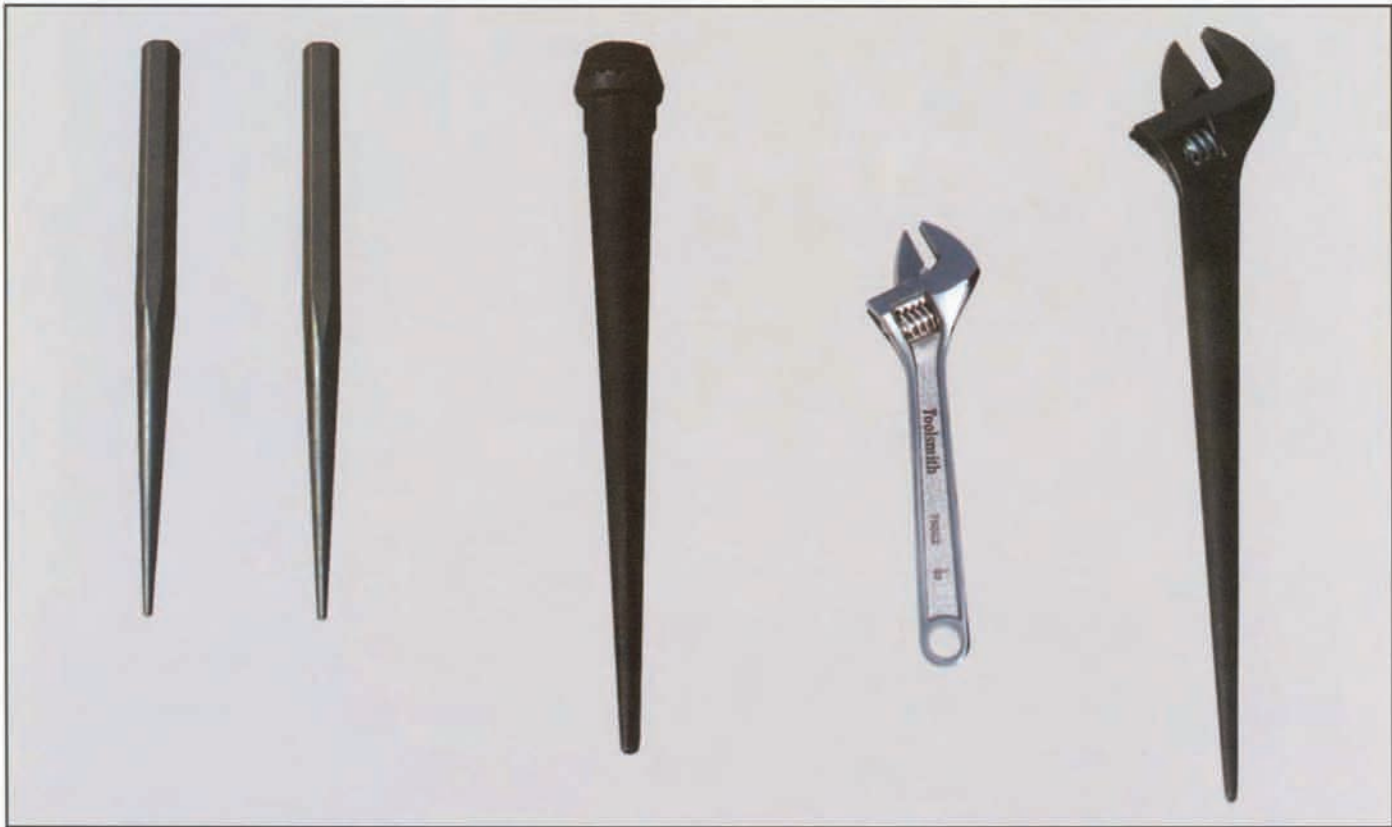
Hole alignment pins Top diameter 5/8" Point diameter. 5/16" Length 11"
