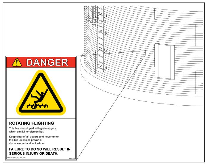
**NOTE:** If the Safety Sign cannot be easily read for any reason or has been painted over, replace it immediately. Additional Safety Signs may be obtained free of charge from the dealer, distributor or ordered from the factory.
