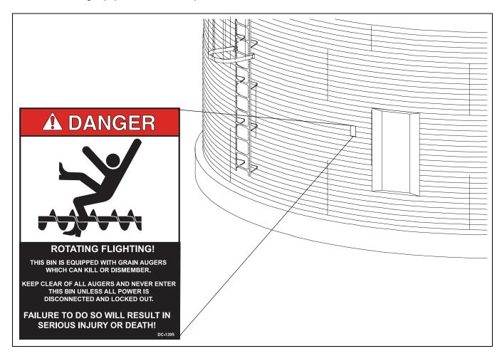
**NOTE:** If the safety sign cannot be easily read for any reason or has been painted over, replace it immediately. Additional safety signs may be obtained free of charge from the dealer, distributor or ordered from the factory.
