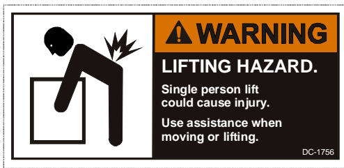
A) DC-1756 Location: Corners of mounting plate Size: 4 3/4" x 2 1/4"
