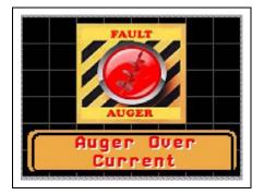
Figure 12A Auger Over Current
