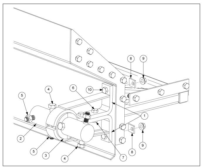
16" Flight Connection Components Parts List
