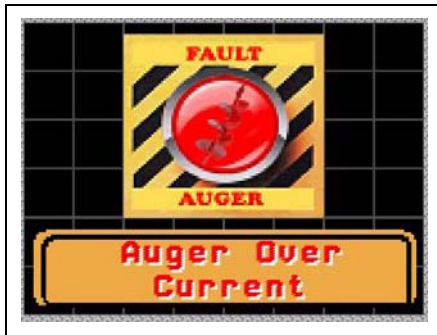
Figure 12A Auger Over Current
