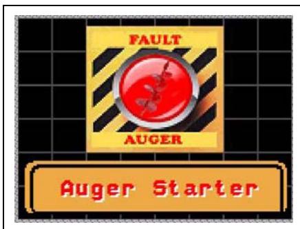
Figure 5Q Auger Starter Fault
