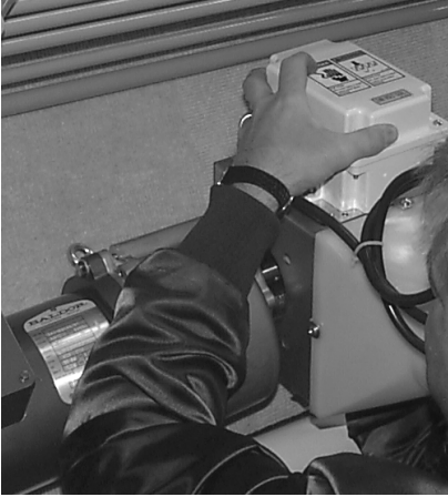
Figure 17: Assembly of the control unit to the drive unit
