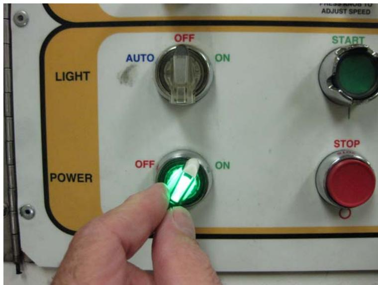
Turn on the Control Power and energize the dryer's control system.
