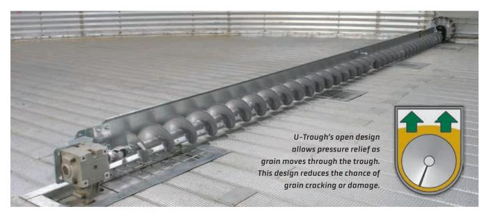
Available for bins up to 78' dia., the U-Trough fits under standard 12" floors, as well as most other aeration floors. It features an adjustable flight for expansion to the outer wall, dual-action sweep wheels move the unloader through grain while sweeping outer sidewall grain, and is designed to help sustain grain quality.
